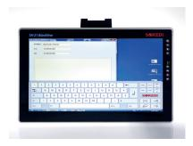
The strong 4 mm anti-glare bulletproof glass layer above the screen withstands acid, cleaning fluids and disinfectants as well as extreme operational demands. Behind the glass there is a projective capacitive touch panel. A special sensitivity control allows for reliable gesture control — and this even when wearing gloves.
