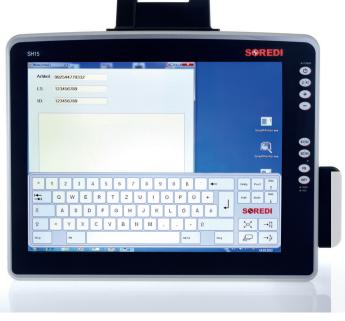
The powerful computer for industry of the series SH in display sizes SH 10, SH 12 and SH 15 offer highly-robust, fan-less PC technology in a completely closed chassis for stationary as well as mobile use.
